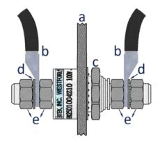
Mounting & Electrode Torque: 50"lbs (5.6Nm)
