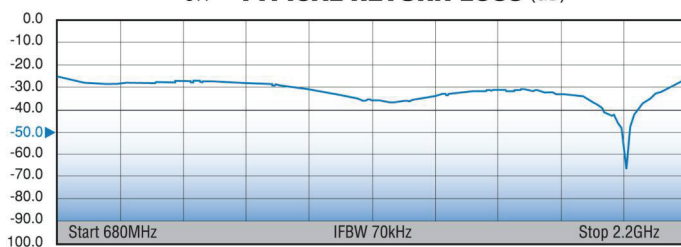
S11 TYPICAL RETURN LOSS (dB)
