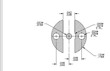
PRINTED WIRING BOARD FOOTPRINT
