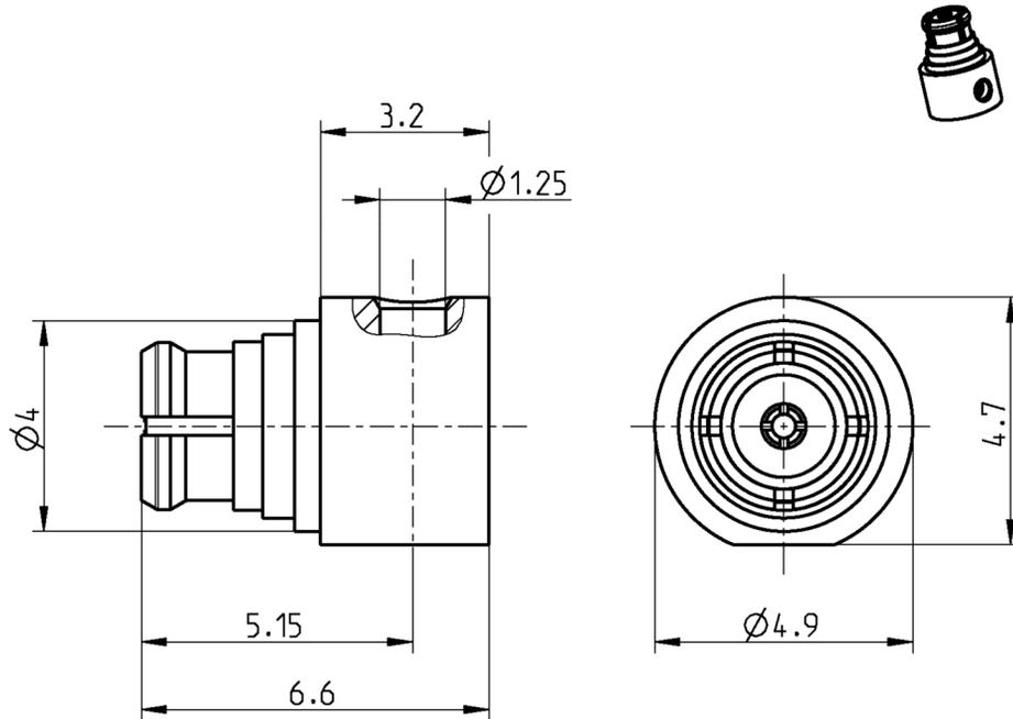
All dimensions are in mm; tolerances acc. ISO 2768 m-H
