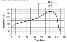
Higher temperature (>260 °C) and longer process duration would permanently damage the switches.
