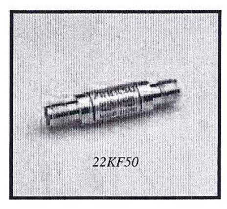
The 22 Series Open/Shorts are used on the test port of an SWR Autotester or SWR bridge to establish a full reflection reference for accurate SWR measurements. When used with scalar network analyzers, the open and short reflections over a swept frequency range can be automatically averaged to enhance measurement accuracy. All models consist of an open on one end and a short on the other.
