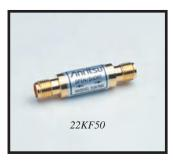
The 22 Series Open/Shorts are used on the test port of an SWR Autotester or SWR bridge to establish a full reflection reference for accurate SWR measurements. When used with scalar network analyzers, the open and short reflections over a swept frequency range can be automatically averaged to enhance measurement accuracy. All models consist of an open on one end and a short on the other.
